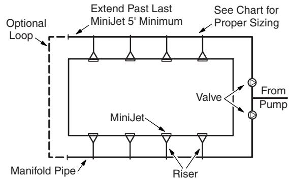
3. When the MiniJets are lined up to project water streams of equal distance, cut the risers to equal lengths. When the MiniJets are not set in lines parallel to the pool edge, valve them separately.
